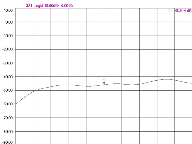
FIG. 7. Vector network analyzer plot showing S21 for the gain antenna. Compare with Figure 4 where the experimental conditions are the same, except now a reflector plane is used behind the NE-2 bulb resulting in a 6 dB signal improvement.
