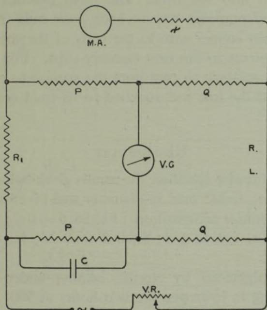
FIG. 1—Kelvin double bridge adapted to A.C. measurements.
