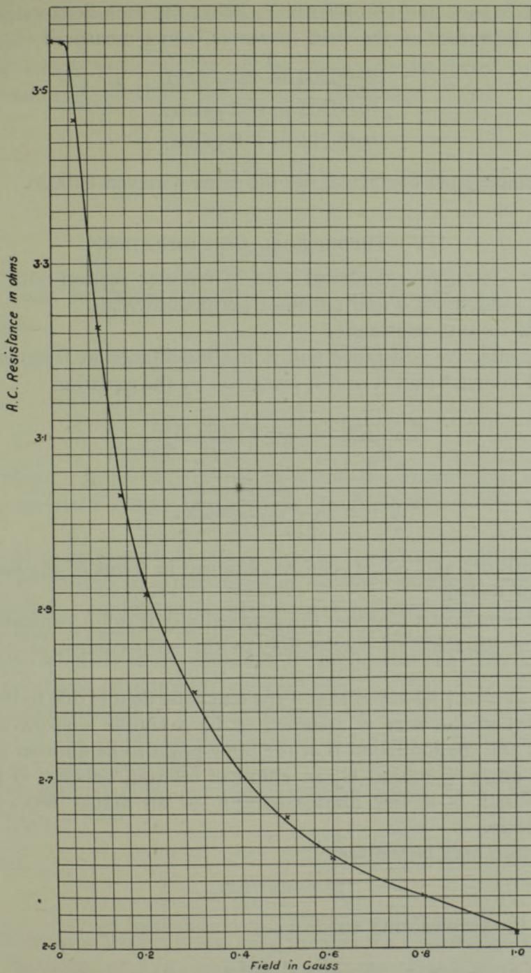
FIG. 6—Variation of A.C. resistance with applied longitudinal field. Frequency 515~, optimum current. Length 15.25 cm.; diameter 0.0183 cm.
