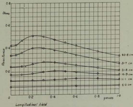
FIG. 5—Variation of resistance and reactance with longitudinal field. Wires of diameter 0.445 cm., and different lengths. Frequency 515~. "Optimum current" 25 m/A.
