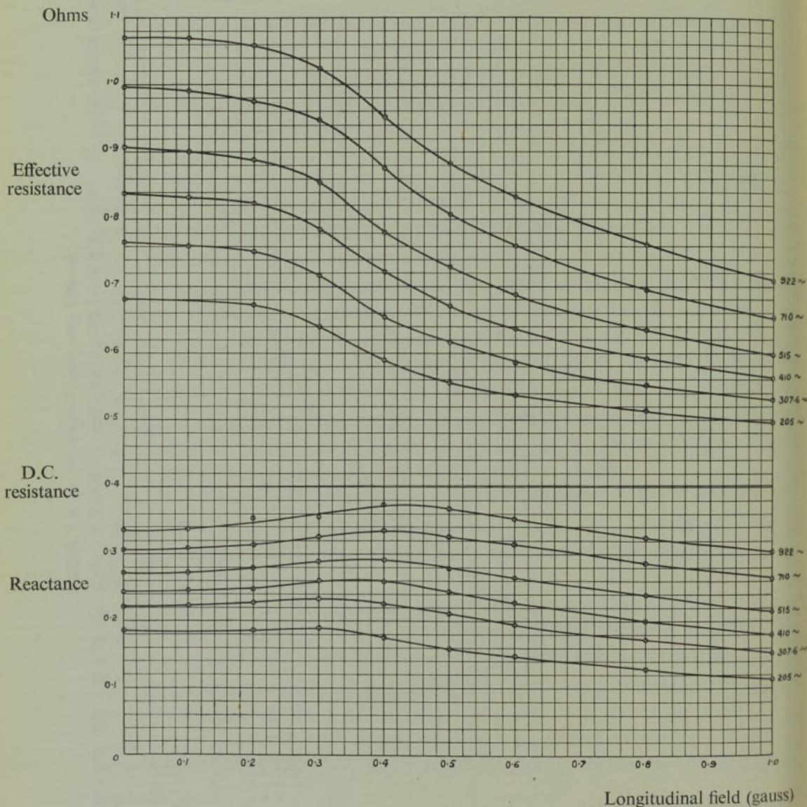
FIG. 4—Variation of effective resistance and reactance with longitudinal field at different frequencies and optimum current. Wire 15.25 cm. long; 0.445 mm. diameter.
