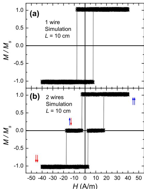
Fig. 4: Simulated hysteresis loop for one and two wires based on the box model.
